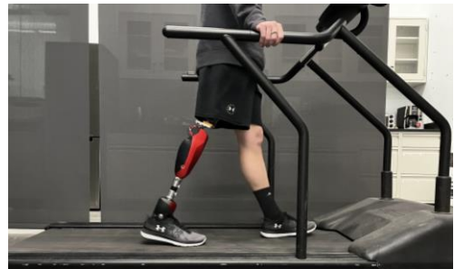
Fig. 5 Side view of participant wearing the Utah Bionic Leg during the experiment.
