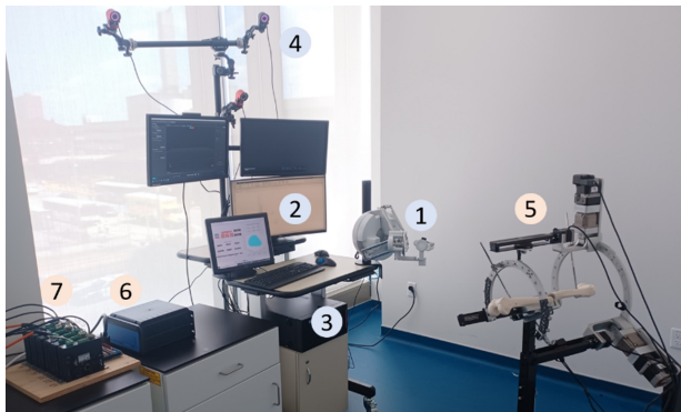
Fig. 11. Robossis system. The haptic unit includes ① the haptic sigma.7, ② screen monitors, ③ the haptic unit PC, and ④ the Optitrack optical trackers. The surgical unit includes ⑤ Robossis surgical robot, ⑥ the surgical unit PC (Speedgoat, Mathworks - Switzerland), and ⑦ motor drivers.
