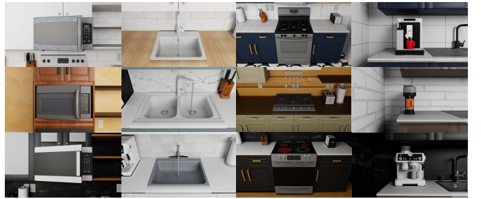
Fig. 4: Examples of Interactable Appliances. Our simulation framework comes with dozens of appliances. Several types of appliances are articulated. For example, we can open and close doors on microwaves and twist knobs on stoves. Some appliances can undergo state changes, e.g. , when we turn the knob on the stove, the corresponding burner turns on.
