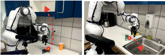
Fig. 9: Real-World Experiment Setup. We conduct experiments in a real-world kitchen environment with a Franka Emika Panda arm on a wheeled mobile platform. The two pictures illustrate two of the three evaluation tasks: (left) pick and place an object from the counter to the cabinet, and (right) pick and place an object from the counter to the sink.
