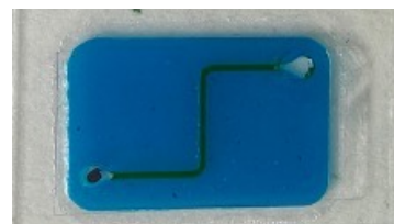
Fig. 3. Printed microfluidic channel test structure using the described flexible cavity fabrication process. The printed structure has been capped with a laminating film and inlet and outlet holes have been punched in the capping layer to allow fluid flow. The cavity has been filled with dyed water to illustrate its functionality as a microfluidic channel.
