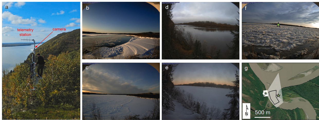
Fig. 3. Shore-based camera installation (a) and ice type examples from shore-based photos: pan ice (b) and rough ice cover (c) on the Tanana R.; skim ice (d) and smooth ice (e) on the Innoko R.; and wet, rough ice on the Kuskokwim River (f). Panel g shows training camera location on the Kuskokwim River (white camera icon) with approximate range of view in white and SAR pixel sampling area outlined in black. Green stars in panels f and g show the same location. Photo credit (a) C. Arp. Background image (g): Alaska High Resolution Imagery RGB 2020 (Maxar Technologies Inc., Alaska Geospatial Office, USGS). (For interpretation of the references to colour in this figure legend, the reader is referred to the web version of this article.)
