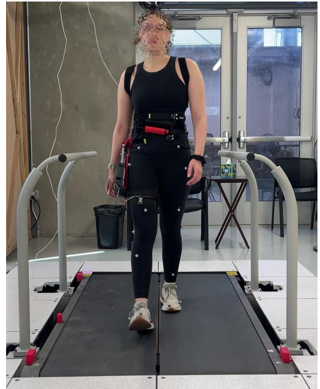
Fig. 10 Subject (S1) walked on an instrumented treadmill at their self-selected walking speed with the powered exoskeleton in a unilateral configuration. Reflective marker trajectories were recorded with Vicon motion capture cameras.
