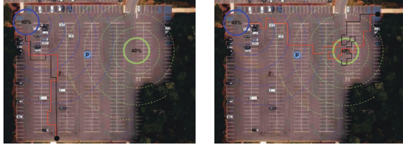
Fig. 10: The field experiment in the parking lot. The two solid line circles in both figures indicate that the only target could be within this region with a 40% probability. The dashed arcs represent the probability field of each region. The black dot is the starting position of the agent. The solid red line is the trajectory of our framework, and the solid black is the trajectory of the single-behavior framework.
