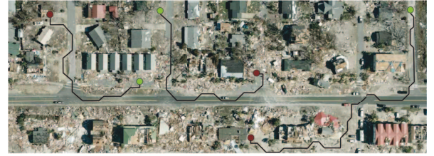
Fig. 6: The trajectories of robots to travel to allocated tasks. The CCQ model is trained in various maps. After training, we use the trained CCQ model to find paths in our post-disaster environment. The red dots are the positions of the allocated tasks, and the green dots are the beginning positions of the robots.
