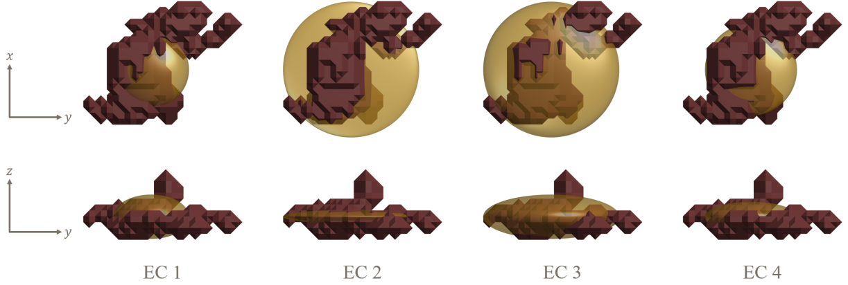
Figure 9: Effect of ellipsoid generation method on the resulting shape of the ellipsoid. A single particle is reconstructed and shown from two directions: the loading direction along the z -axis (top row) and perpendicular to the loading direction (bottom row). The ellipsoid that results from each of the four options is shown for the particle, where the numeric identifier corresponds to the options as listed in Table 1.
