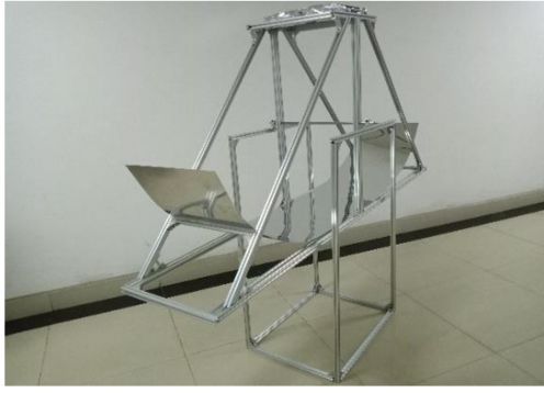
Fig. 9 (b). A prototype of the concentrated PV system.
