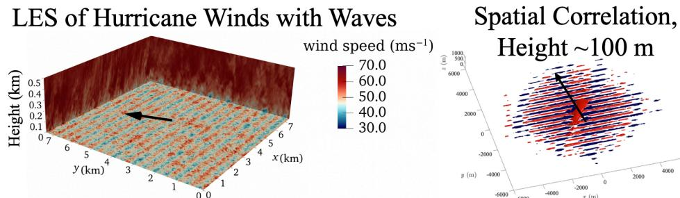
Left: Wave-resolving large-eddy simulations of hurricane winds. Right: 3D spatial correlation of turbulent eddies in hurricanes; red (blue) shows positive (negative) correlations. The black arrow shows the direction of the mean wind velocity vector.
