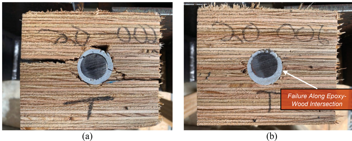
Fig. 9. (a) Splitting of MPP and (b) separation at adhesive-wood intersection. Sections taken at one-half of specimen embedment depth (254 mm for shown specimen).
