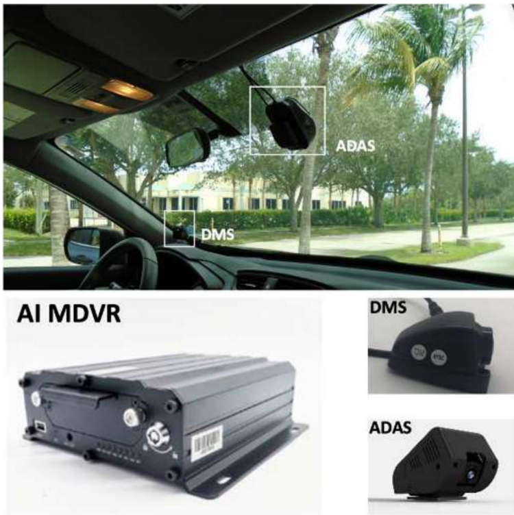
Fig. 3 In-Vehicle Vision Sensors, 2 Cameras + MDVR
