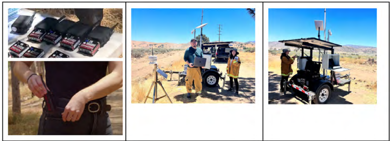
Fig. 3. The figure shows sensor deployment at the prescribed burn site: the left image displays body-worn sensors, the middle image shows the Gateway sensor unit mounted on a tripod with the UCSD team setting up the edge compute laptop, and the right image features the trailer unit equipped with a 3D wind sensor, solar power, a 24+ hour battery, and satellite internet.
