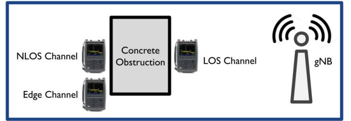
Fig. 3: Experimental Setup for LOS, Edge, and NLOS Wireless Channel Situations [21].
