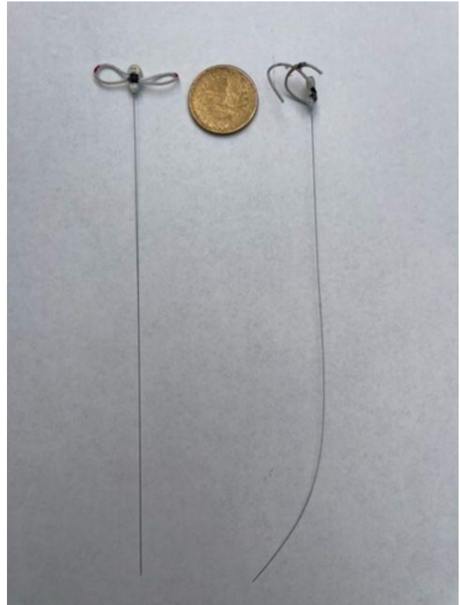
Fig. 1. Example of how longer antennas (in this case, 18 cm) may curl or become hooked over time (right) relative to their appearance at deployment (left). This curled or hook-like shape may increase the likelihood of tagged birds becoming entangled in vegetation and other parts of their environment.
