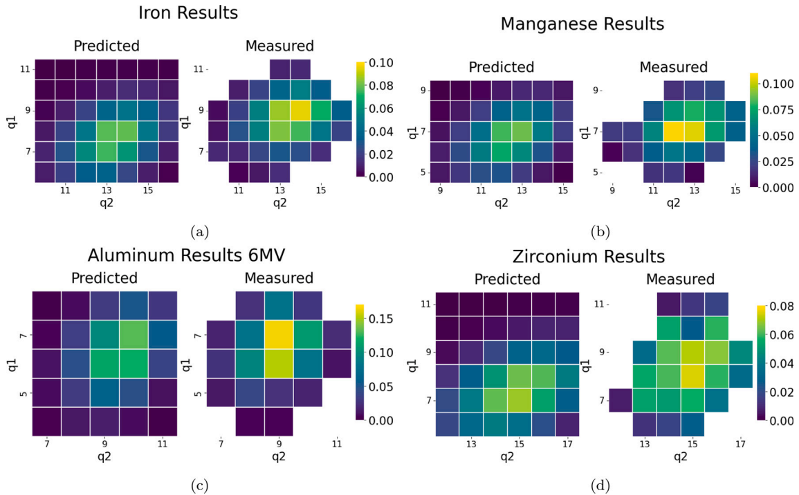
Fig. 4. Observed second foil stripping charge state distributions and their predicted values. Each state was measured until the final beam current was imperceptible on the final Faraday cup. The observed dip in the \text{Zr}^{10+ \rightarrow 15+} plot exhibited the same behavior upon remeasurement. The color scale denotes what fraction of the total transmission ( \epsilon_D defined in Eq. (12) and listed in Table 1) each state occupies.
