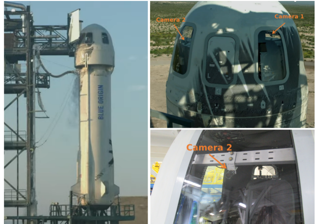
Fig. 6. Sub-orbital rocket on launch pad used for data collection (left). Close view of camera mounted inside the capsule window (bottom right) and a view of both cameras inside the capsule before launch (top right). Images courtesy of Blue Origin.
