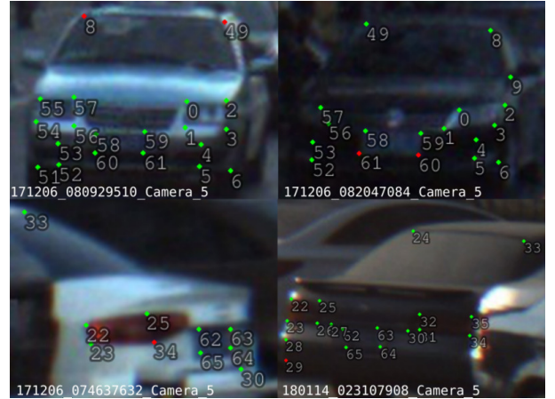
Fig. 9. We pass ground-truth annotated keypoints to ROBIN, using a winding order dictionary generated from ray tracing. Green dots represent keypoints inliers accepted by ROBIN. Red dots represent outliers rejected by ROBIN. In these four examples, ROBIN correctly rejects mislabelled keypoints. From top left clockwise: #8 and #49 are switched (with respect to the CAD models); #61 and #60 are switched; #34 is wrongly placed (should be #26 instead); #29 is wrongly placed (should be placed below the right tail light).
