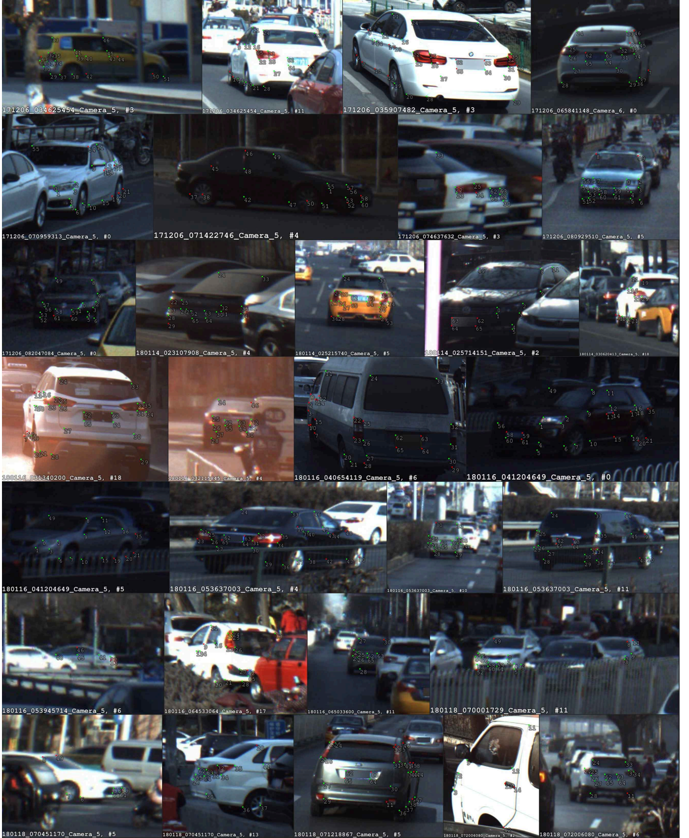
Fig. A7. Mislabeled ground-truth keypoint annotations in ApolloScape detected by ROBIN. Green and red dots represent inliers and outliers determined by ROBIN, respectively. For a detailed description of the incorrect keypoint annotations for each image, we refer the reader to Table A4
