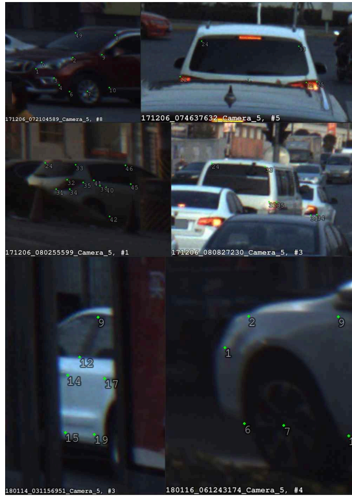
Fig. A9. Mislabeled ground-truth keypoint annotations in ApolloScape that were not detected by ROBIN. Green dots represent inliers determined by ROBIN. For details, we refer the reader to Table A5
