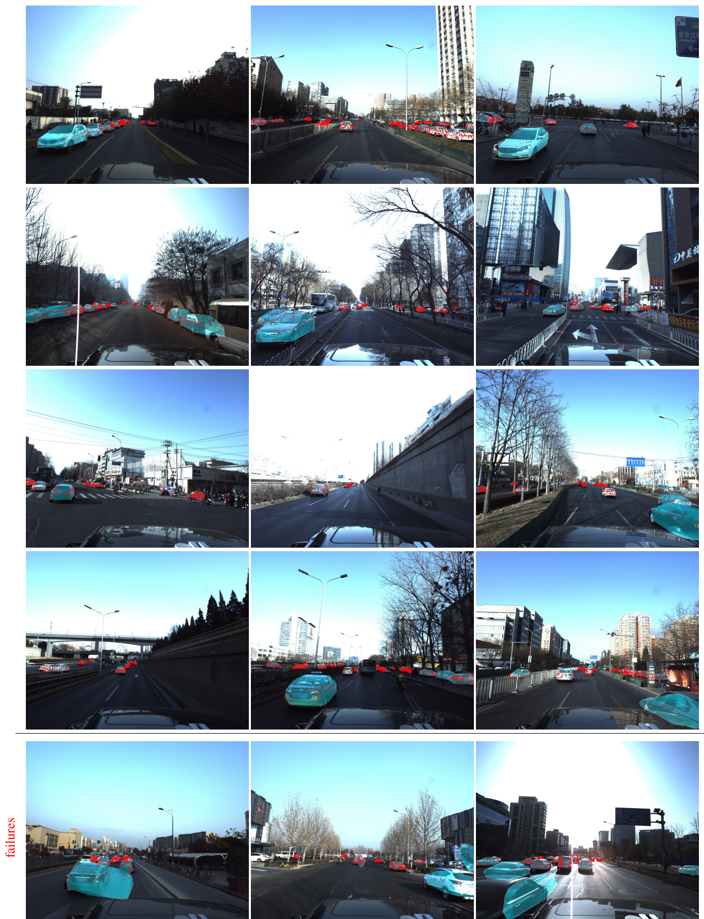
Fig. A6. Qualitative results for PACE3D#: overlay of estimated vehicle pose and shape on the images from the ApolloScape dataset. The images are manually selected out of the validation set in the dataset to showcase successful vehicle localization (top 4 rows) as well as failure cases (last row).
