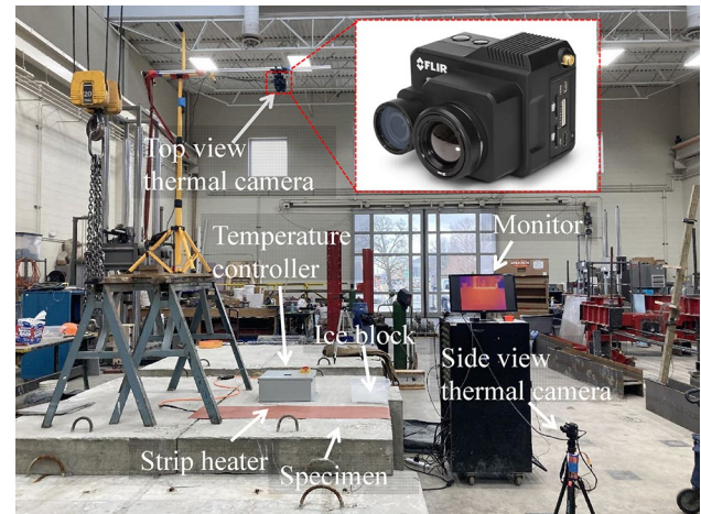
Fig. 5 Active IRT test setup
