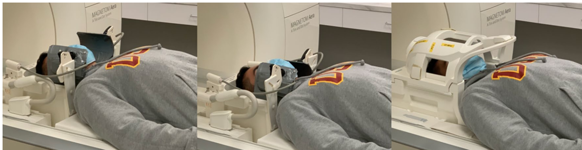
Fig. 3 Custom upper airway (UA) and prototype head–neck (HN) coil for 0.55 Tesla MRI. (Left) 8-channel UA coil before adjustment of coil elements. (Center) UA coil with coil elements placed as close as possible to the upper airway region without contacting the skin or otherwise altering speech production. A 9 th element can be placed in
