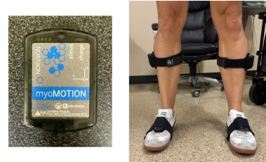
Fig. 1. Noraxon Myomotion IMU and Placement on Lower Body
