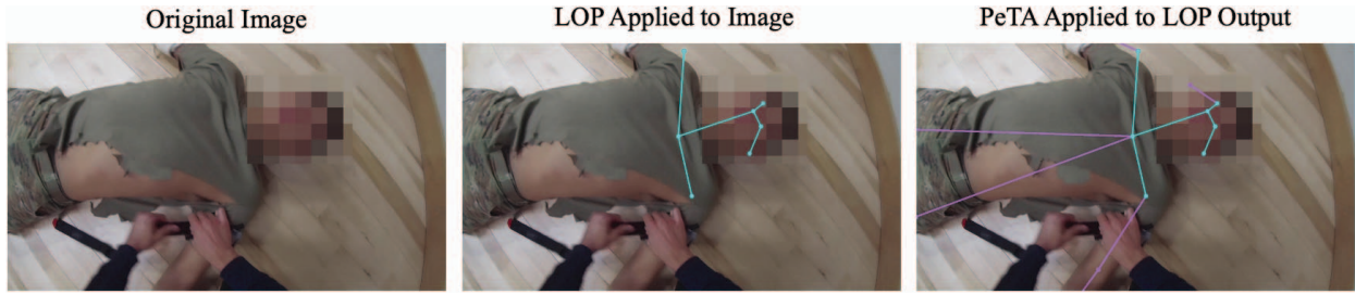
Figure 5. An example of the application of our Pose-Enhancing Transformation Algorithm (PeTA). From left to right, this figure shows the input image, the image following the application of the Lightweight OpenPose (LOP) [21] algorithm, and finally the image after using PeTA to infer the missing joints. Note that the face is blurred for the purposes of this paper, but is not blurred for LOP or PeTA algorithms.
