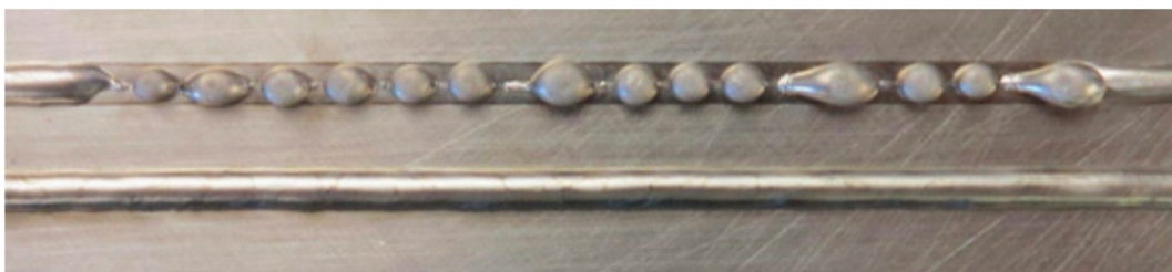
Figure 33. Top track deposited without employing a controller. The bottom track deposited utilizing a controller for adjusting the position of the deposition head in the Z direction (reproduced with permission from [97]: copyright 2014, Elsevier Ltd.).
