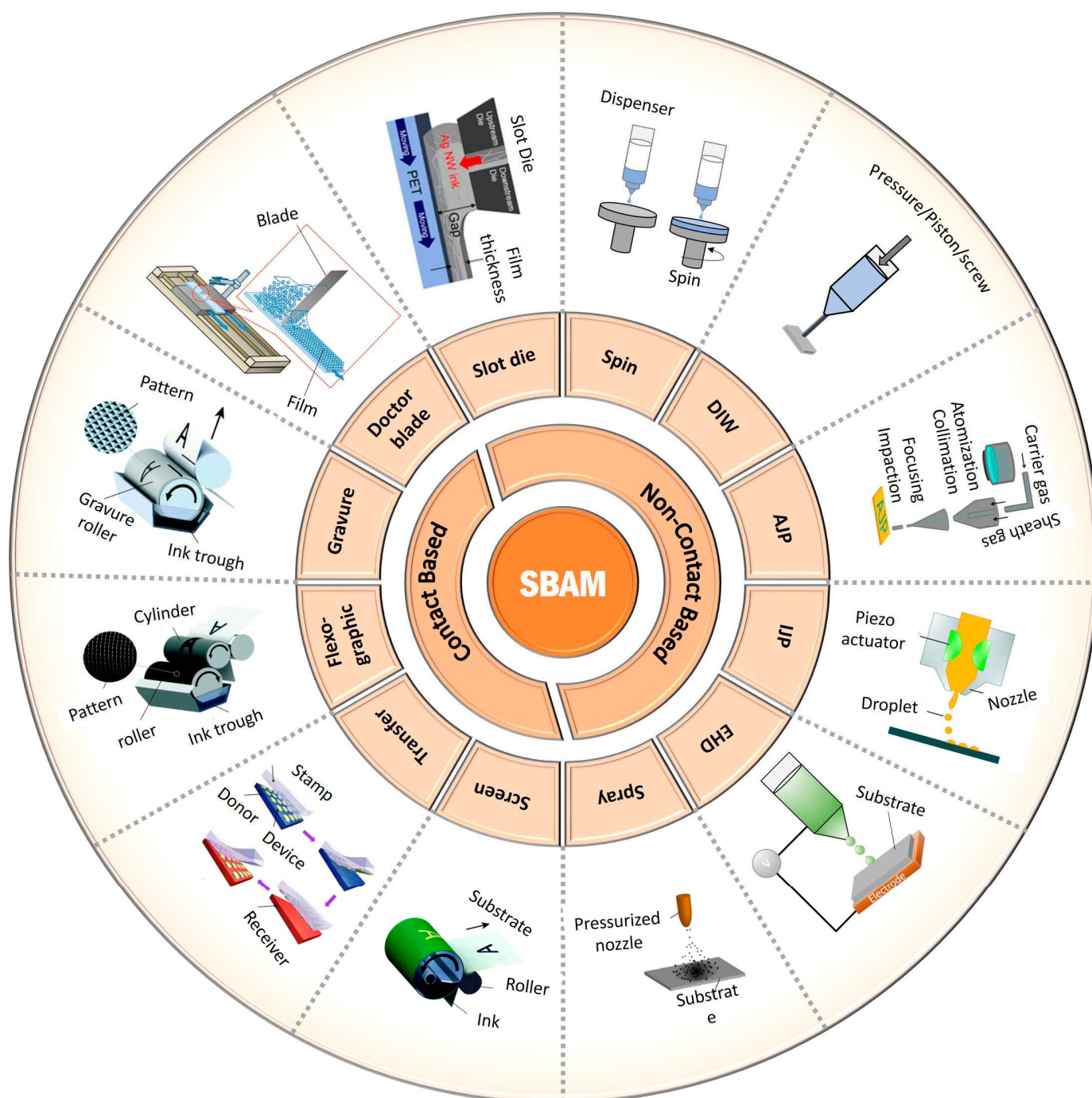
Figure 1. Contact and non-contact solution-based additive manufacturing techniques (schematics of printing methods adapted or reproduced with permission from [66,83–88]: copyright 2021, Elsevier Ltd.; copyright 2018, Royal Society of Chemistry; copyright 2020, Royal Society of Chemistry; Copyright 2010, American Chemical Society; copyright 2019, MDPI; copyright 2018, IOP Publishing; copyright 2016, Nature Publishing Group).
