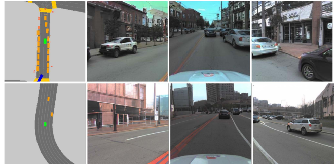
Fig. 1. Proposed BEVGen model generates realistic and spatially consistent street-view images from BEV layout. There are 3 camera views surrounding the ego vehicle as indicated by the green rectangle in the BEV layout.
