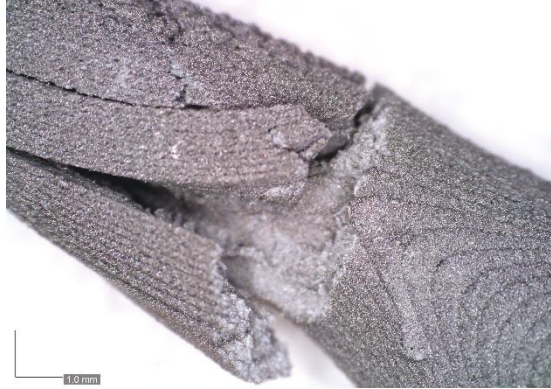
Fig. 8: Torsional fracture response of Sample 1
