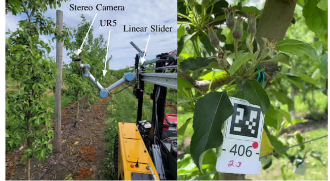
Fig. 1. Left: Stereo camera attached to a 7 DoF robotic arm. Right: Example of a fruitlet cluster with AprilTag hung in close proximity for identification.
