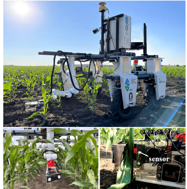
Fig. 1. Robot inserting sensors into cornstalks to monitor plant nitrate concentration in Curtiss Farm, Iowa. Our custom gripper utilizes contacts in a clutter-rich environment to precisely align with stalks and insert sensors.
