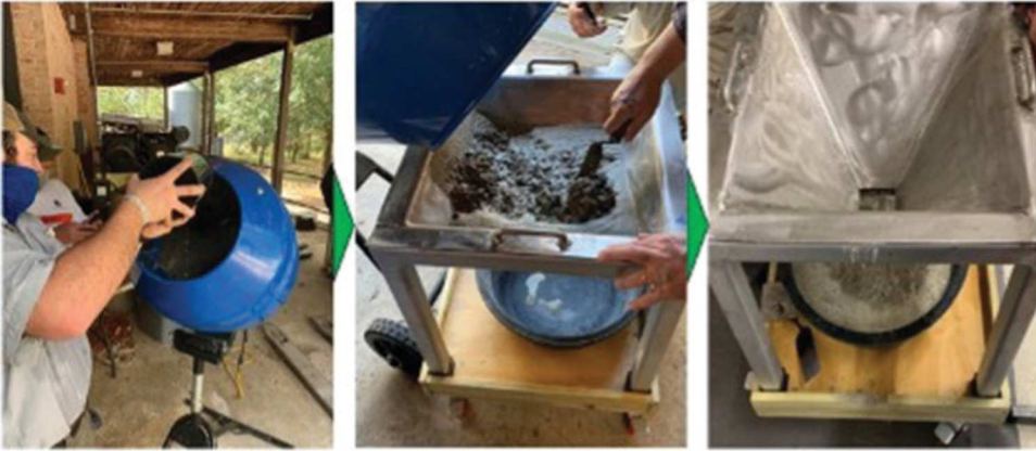
Figure 1. Procedure of concrete batch production – ingredient mixing, followed by pour into hopper, followed by release into circular plastic container and rinsing.
