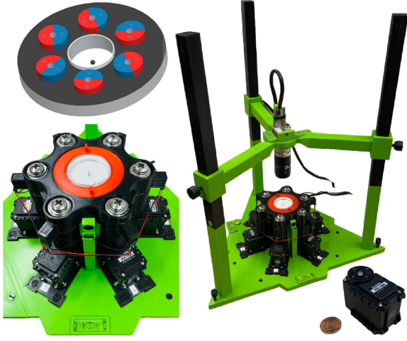
Fig. 1. Experimental setup adopted from [4] with modifications in the size of magnets, design of camera mount, and inclusion of a rigid base structure. This magnetic manipulator (bottom left) utilizes 6 diametrically magnetized cylindrical permanent magnets that can freely rotate a full 360^\circ inside their guiding cylinders using 6 independent servomotors (bottom right).
