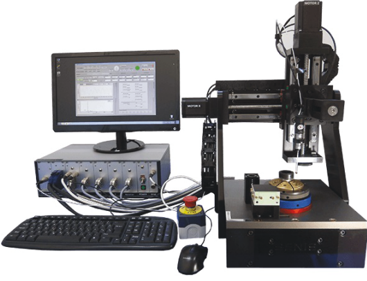
Fig. 4. Senis MMS-1A-RS magnetic field scanner. This instrument provides a platform for measurement and empirical modeling of magnetic fields. It consists of a holder for accommodating magnets, a 3D manipulator which can scan a volume of 135 \times 135 \times 135 mm around the magnets with 1 \mu\text{m} spatial resolution, and a 3D magnetic sensor on the tip of the manipulator, which can measure a vector of magnetic field with 0.1% accuracy.
