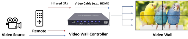
Figure 1: Architecture of a representative video wall system.
