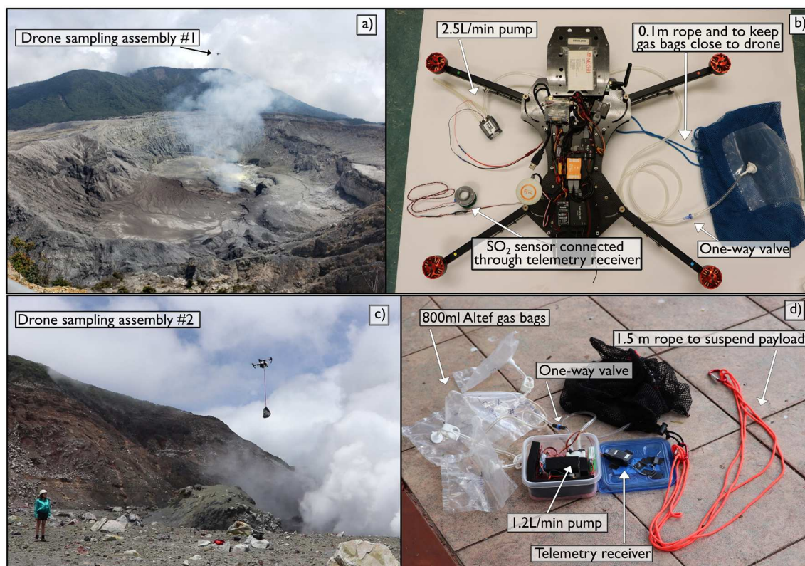
Fig. 2. Sampling assembly by UAS used at Poás in April 2019. a) Distal assembly used for sampling the volcanic plume on 25 April b) Distal assembly components and specifications. c) Proximal assembly used for sampling at Poás crater on 30 April 2019. d) Proximal assembly components and specifications.
