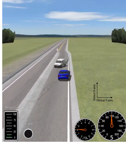
Figure 12.: Collision-avoidance scenario in CarSim. In this scenario, the oncoming vehicle (the white van) enters the opposite lane, and the host vehicle (the blue van) performs an evasive maneuver to avoid a collision.
