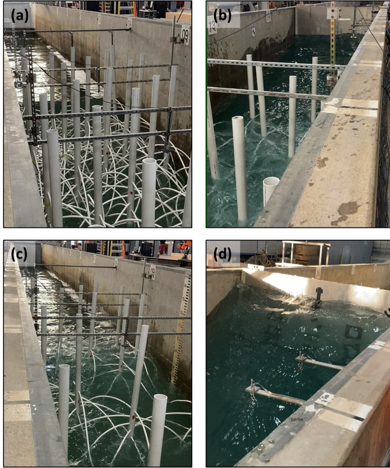
Figure 6: Photographs of wave-mangrove-wall interaction: (a), (b) high-density (HD) configuration for (a) h_v = 0.73 m, view through forest section towards the wave maker and (b) h_v = 1.85 m, view of wave-wall interaction; (c), (d) low-density (LD) configuration for (c) h_v = 1.03 m, view through forest section towards the wave maker and (d) h_v = 1.85 m, view of wave-wall interaction.
