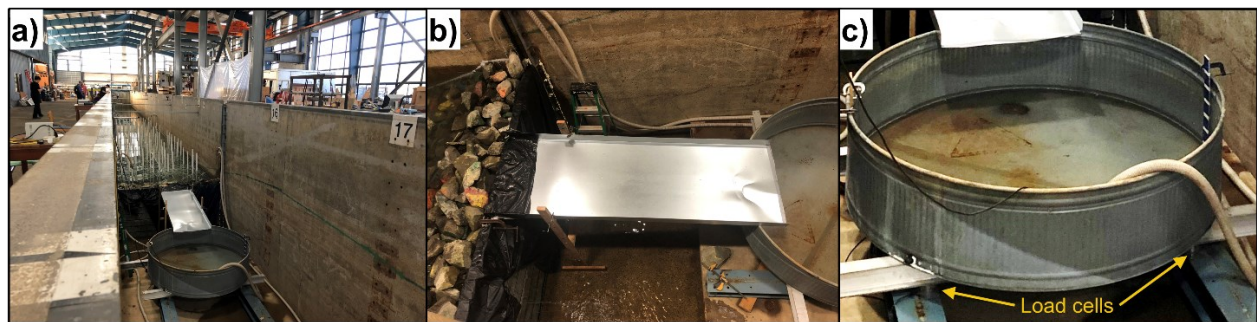
Figure 6. Overtopping catchment system. (a) View of test setup showing wavemaker (back) to overtopping basin (front). (b) Secured tray directing water into the basin. (c) Overtopping catchment basin with two of the four load cells indicated.
