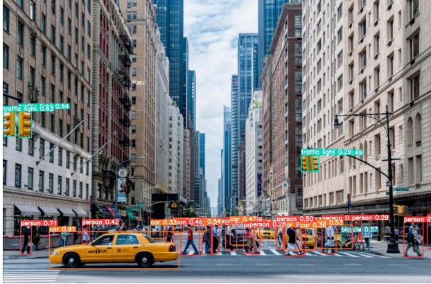
Fig. 2: An example of an input frame for an autonomous vehicle application, where the objects of interest are defined as people, cars, traffic lights, street lanes, etc
