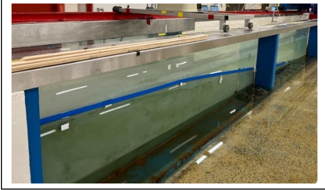
Fig. 4. Photograph of Sediment Flume with 1:10 Slope Marked in Blue Tape
