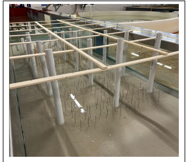
Fig. 7. Photograph Showing 50% R. mangle , 50% A. germinans Mangrove Forest Test Configuration
