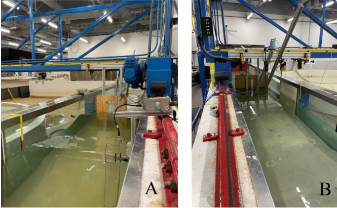
Fig. 1. A: View from wave maker showing wave propagation toward wall installed in tank, B: Rear view wall showing method for affixing wall to bridge
