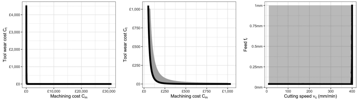
Fig. 7 Left: image (gray) and PF (black) of the single cut turning cost operation biobjective function. Middle: the left plot zoomed into the lower-left region. Right: input space (gray) and PS (black).
