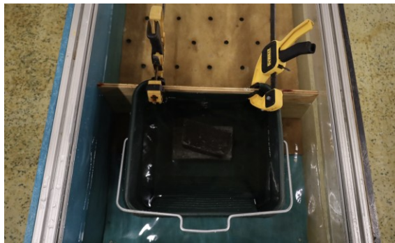
Figure 5: Wall and Overtopping Basin for 1:8-scale Experiments
