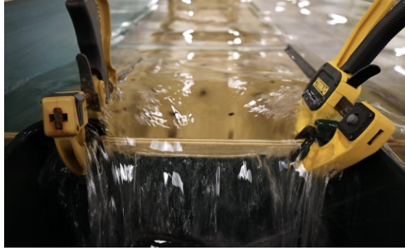
Figure 7: Waves Overtopping the Wall into the Collection Basin during Baseline Condition
