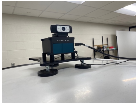
Figure 2. Data acquisition setup: a high-definition 1080p Logitech webcam mounted above a Livox LiDAR with a 120-degree horizontal field of view, both installed on top of a vehicle to gather spatial and video data.
