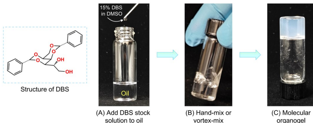
Figure 2. DBS organogels and their preparation by a simple new method at room temperature. The structure of DBS is shown in the box. To make the gel, a stock solution of 15% DBS in DMSO is first prepared by simply mixing the two at room temperature. (A) The oil to be gelled is then taken in a vial (here it is 2 g butanol). The stock solution (0.14 g) is added such that the DBS concentration in the mixture becomes 1%. (B) The sample is then mixed by hand or using a vortex mixer for a few seconds. (C) Right afterward, the sample becomes an organogel due to the self-assembly of DBS into a nanofibrillar network. This method to form DBS gels is simple, quick and does not require heat. It is also shown by Movie S1.
