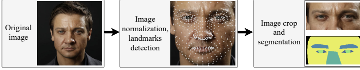
Fig. 7. Preprocessing of a sample from the CelebAMask-HQ dataset: face and face landmarks are detected for image normalization and eyes' region image crop and segmentation.
