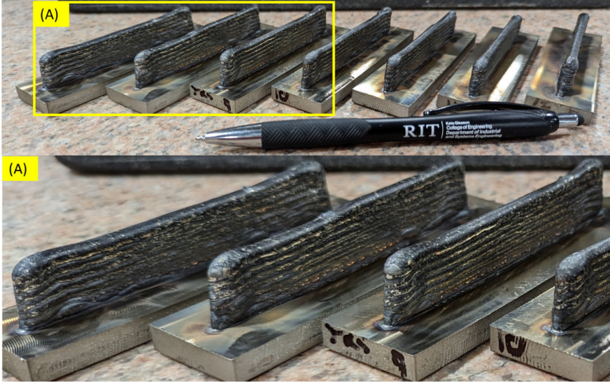
Figure 16: Seven thin-wall parts ( 150 \text{ mm} \times 2 \text{ mm} \times 10 \text{ mm} ) consisting of 10 layers deposited with processing parameters corresponding to the stable regime ( P = 1500 \text{ W} , V = 500 \text{ mm} \cdot \text{min}^{-1} , E_L = 180 \text{ J} \cdot \text{mm}^{-1} ). All seven parts were completed successfully.
