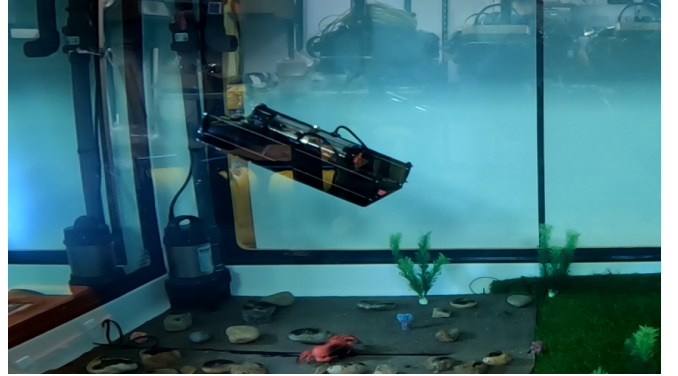
Fig. 1: ReefGlider shown here in a tank is a highly maneuverable underwater robot that uses buoyancy for propulsion, but unlike other gliders is highly maneuverable.
