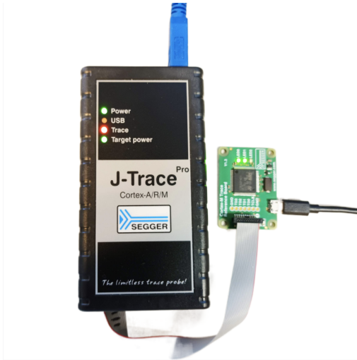
Fig. 1. Fuzzing Trace Reference board STM32F407VE firmware with J-Trace Pro debug dongle [12]
