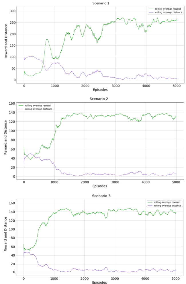
Figure 3: Rolling average reward and distance of ego vehicle to a destination during training for 5000 episodes in each scenario. The green curve represents the rolling average reward of the past 100 episodes while the blue curve represents the average distance.
