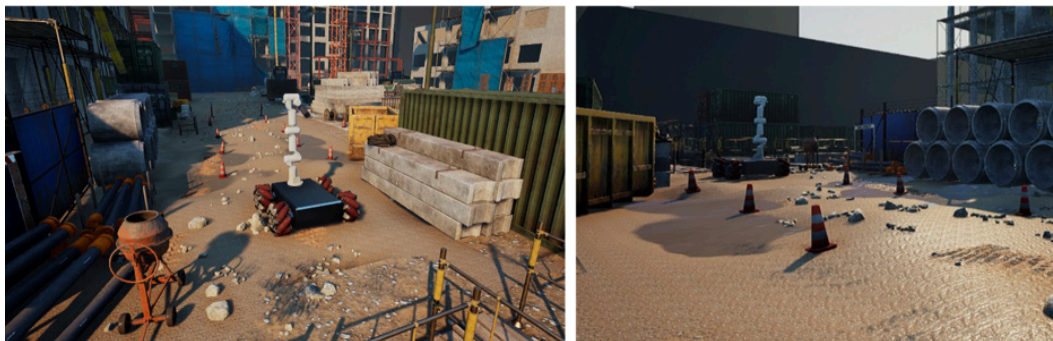
Figure 4. Simulation of a 6-axis robotic arm navigating through a VR-based construction environment
